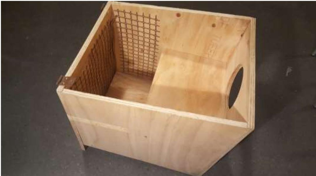
7. Attach roof to hinges and secure down with gate latch hooks. The hook shown has a spring catch, but plain ones are fine as long as there is some tension to prevent them opening when not wanted.
