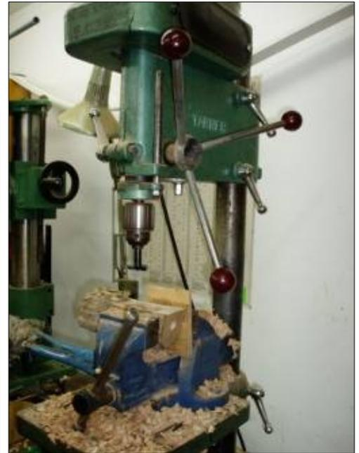
The central cavities are drilled using a drill press (above). We used a 35 mm tungsten tipped Super End Mill bit with 8 mm shank. The holes are drilled in line to create a chamber and any wood remaining can be chiselled out to give a roughly rectangular chamber.
